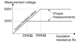
The actual measurement voltage as the function of the measured insulation resistance  $R_x$  (for the maximum measurement voltage).
